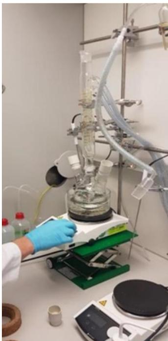
**Figure 3.1:** Experimental setup for the preparation of PS NPs by surfactant-free emulsion polymerization. This picture was taken by Dr. Reza Mohammadi at prof. Dr. N. Vogel's lab at the Institute of Particle Technology, Erlangen, Germany.
